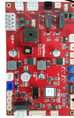
TWOCS6 Cuppillar pcb Replacement (UIID PCB)
