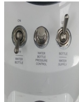
Switch Position After cleaning is complete
